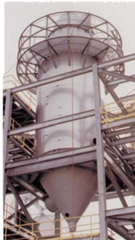
*This spray dryer uses pressure nozzles although the slurry is very abrasive. The tight particle size distribution was required to improve quality and energy efficiency of a downstream process.*
